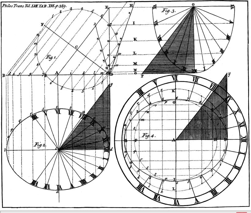
XXXVI. A new Method of constructing Sun-Dials, for any given Latitude, without the Assistance of Dialing Scales or Logarithmic Calculations. By James Ferguson, F. R. S.
